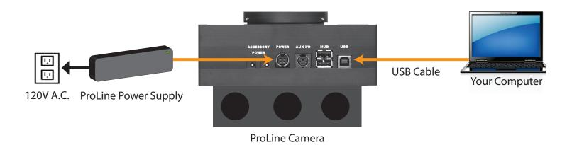
Setup the components as described in the procedure below.
