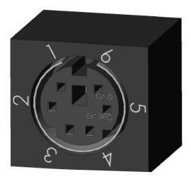
Pin 6 is the electrical ground. Pin 5 is the logic input for the external trigger. (This input has a 22.1K pullup resistor to +3.3V). The external trigger can be setup for either rising edge or falling edge trigger.
