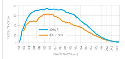
**READ NOISE:** The read noise of the KL6060 FI is 1/3 the noise of the KAF-16803 running at 8 MHz (about 3 second readout time), but the KL6060 FI delivers 19 frames per second.
